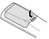
(2) Set three R6P/AA batteries in the battery compartment in the indicated direction.
